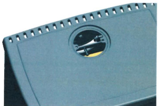
Fig 4.6 Install the cover at the back side
