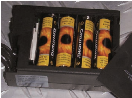
Replacing the batteries of the receiver
