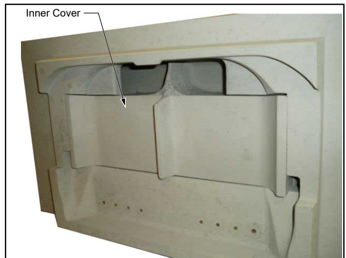
Figure 3.11 - Remove inner cover.
