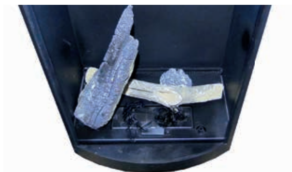
Place log 01 (L) on burner port BP 1. Pay attention that the log slides all the way over the burner port.
